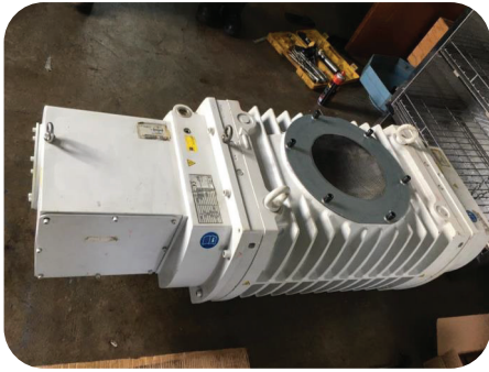
Overhaul Vacuum Pump
