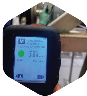
Vibration Monitoring For Installed Rotating Equipments
